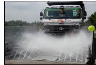
TRUCK WHEEL WASHING SYSTEM
